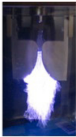
Gliding arc discharge
